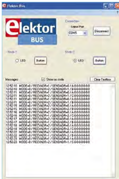
Figure 5. Screenshot of the PC software in action. Our mini-controller can switch the LEDs on the nodes and also show all the messages being sent on the bus.
